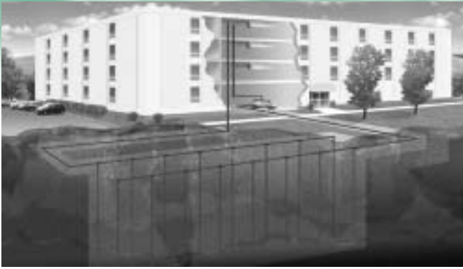
Geothermal Closed Loop
