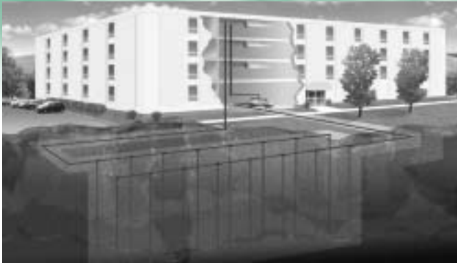
Geothermal Closed Loop
